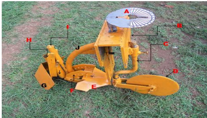
Figure 1: Manure injector components
