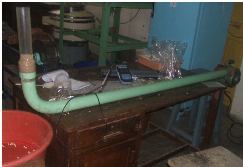
Fig. 2. Experimental set for measuring terminal velocity of drumstick seeds
